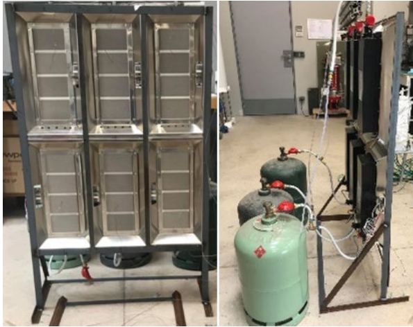
Figure 3: The radiant panels and its gas supply system
